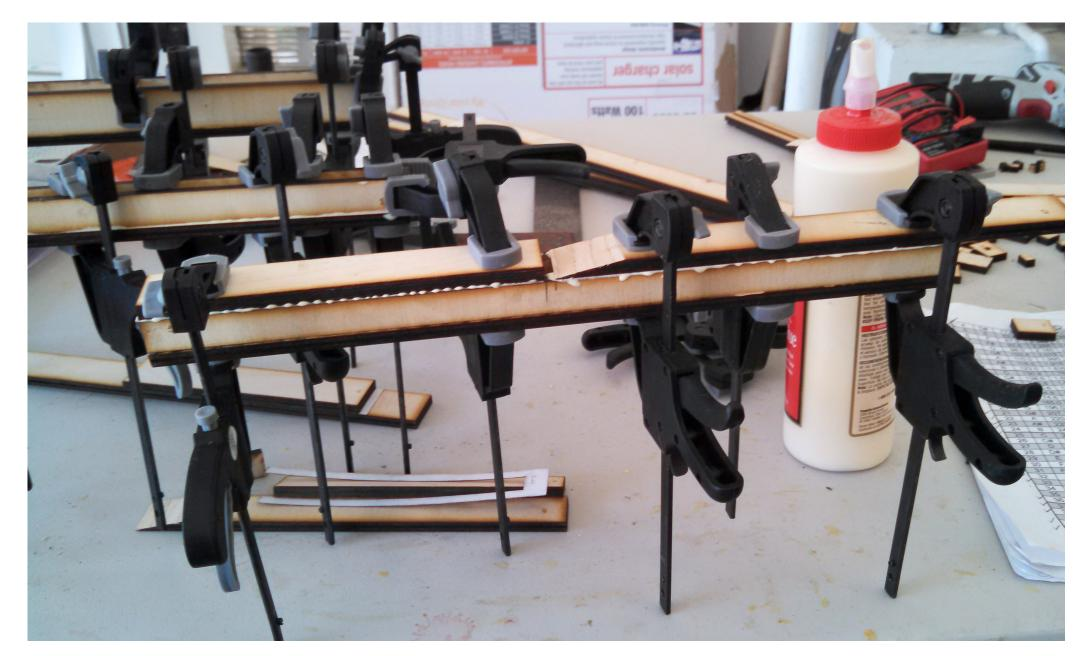
The pipe is thoroughly clamped and left to completely dry. Sometimes the pipe is made a bit long on purpose. The open end of the pipe can then be cut down to the exact length specified by the equations.
