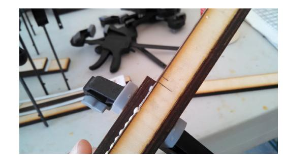
Locate and check the measurement of the marks we made back in step 1. There should be two marks on one of the sides. One mark should line up with the *languid*. The other is called the mouth height mark.
