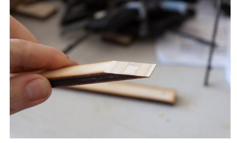
The *upper lip* is the final piece to glue. It tapers down to an edge. This tapered edge is placed along the *mouth height* mark.
