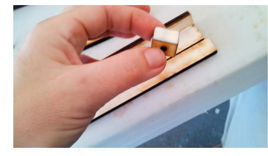
Next, glue the *foot* piece in place at the bottom of the pipe. We used two pieces glued together to make a thick foot. The hole for the air to enter can be seen right above my thumbnail.
