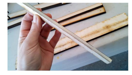
Put a layer of glue on the *side* piece. Make sure it's smooth so the seam will be as air tight as possible.
