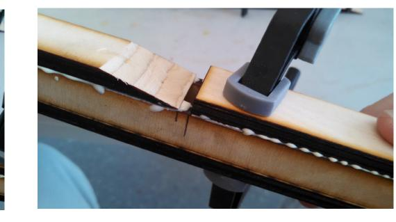
Place the *upper lip* so that the edge lines up with the *mouth height* mark we made. There will be a gap between the tapered end of the *upper lip* and the languid. This gap is called the mouth *height* of the pipe.
