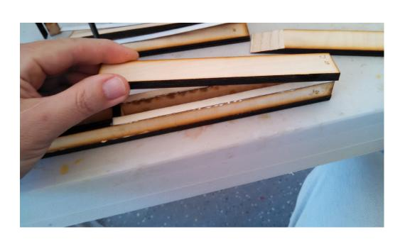
Then we fit the *cap* on top of the gasket. Now we have a box where the wind comes in through the hole in the foot, and out through the wind gap. Where does it go next?
