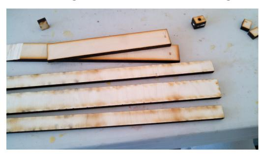
Here's all our parts! Using a spreadsheet and equations from books, we laser cut all the parts for each pipe from one-quarter-inch thick birch plywood.
