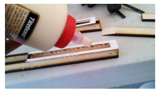
After our gasket dries, we need to put the cap on. We put another layer of glue on top of the gasket.
