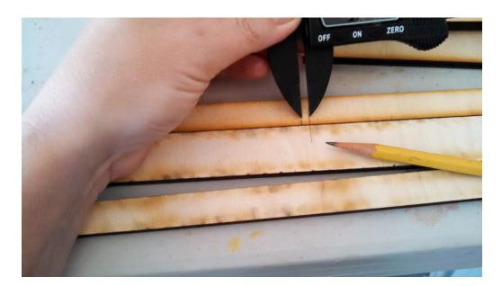
On the side piece with the pencil mark, we measure an additional distance called the *mouth gap*. We add a second mark at that point.
