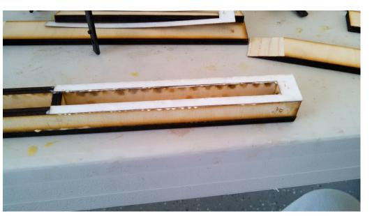
Here is the gasket drying in place. It covers the *foot* and the *sides* that are covered by the *cap*. It doesn't cover the languid, and that space is what makes the wind gap.
