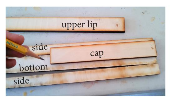
Using the cap piece, we mark a pencil line across the bottom and one of the sides. We want the *languid* to line up with the *cap* piece.
