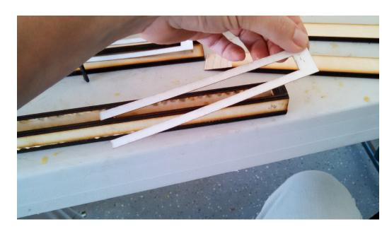
We laser cut the gaskets to match the dimensions of each pipe. These are made from thick paper. We put glue on the gasket and carefully glue it in place.
